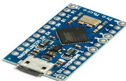
Gambar 1. Arduino Mikro Pro Atmega 32U4
