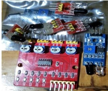
Gambar 3. Sensor Infrared (IR Obstacle)
