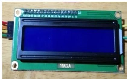
Gambar 4. LCD (Liquid Crystal Display)
